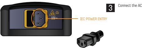
Connect the AC power cable to the IEC POWER ENTRY.
